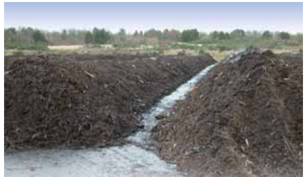
'Windrow' type, Industrial Composting Site
